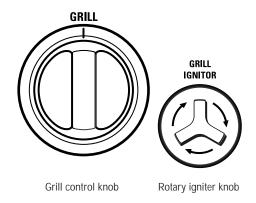
Each grill burner has its own rotary igniter. The igniter knob is located to the immediate right of the control knob.
